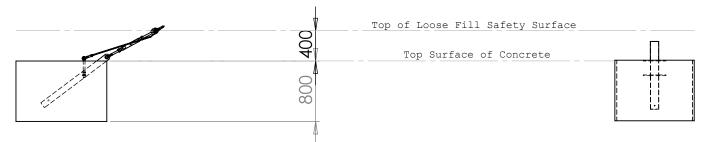
It is important to maintain 400mm between the finished surface level of the safety surface and the top surface level of the concrete. Once the correct position of the holes has been marked prior to excavation, The use of a datum peg is recommended in order to easily relocate the exact foundation position (both horizontally and vertically) which was originally established during setting out.
